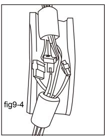
4 shown in the picture, use a piece of thermal insulating jacket to enclose the wiring terminals and sponge. Then glue the thermal insulating jacket and fasten it with cable ties.
