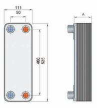
A measure mm = 10 + (2.35 \* n) (+/-2 %)Weight\*\* kg = 2.6 + (0.19 \* n)(n = number of plates) \* Excluding connections
