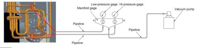
Step 3: Open the valves at both the high-pressure and low-pressure sides and then start the vacuum pump until the gage reading is below -1bar. After that, let the vacuum pump lasts for another 0.5~1.0 hour.
